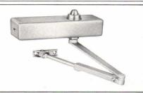
Tested to ANSI specification A156.4-1972, the closer was doormounted under a static load and activated every 4 to 6 seconds over an eight month period. In post-cycling, static tests, it functioned flawlessly in every area of operation: range of checking control; adjustable closing speed; closing force; closing efficiency and cylinder operations. Qualified in every respect as an ANSI Grade I door closer. Ever-enduring cast iron alloy body.
